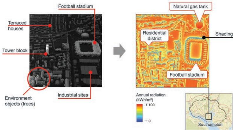
*Figure 15.* LiDAR (left) and in-plane solar radiation (right) results of an example area in Southampton.
