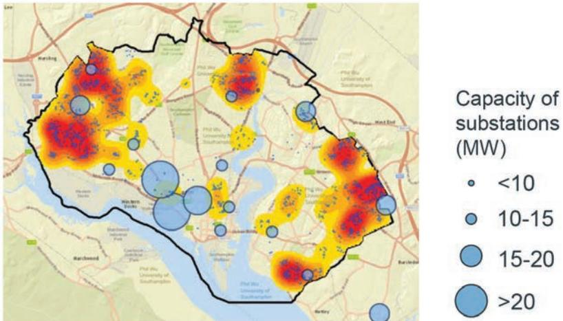
*Figure 16.* Suitable Southampton City Council buildings for rooftop PV deployment as estimated by model and capacity of power sub-stations in the city.
