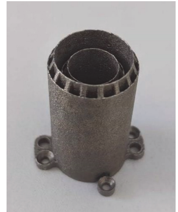
Straight cylinders: first design in 316L (left) and current design in Nickel alloy (right)
