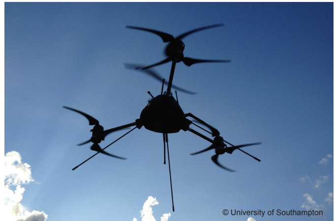
The HALO (2.5 kg) Co-Axial Y6 UAS
