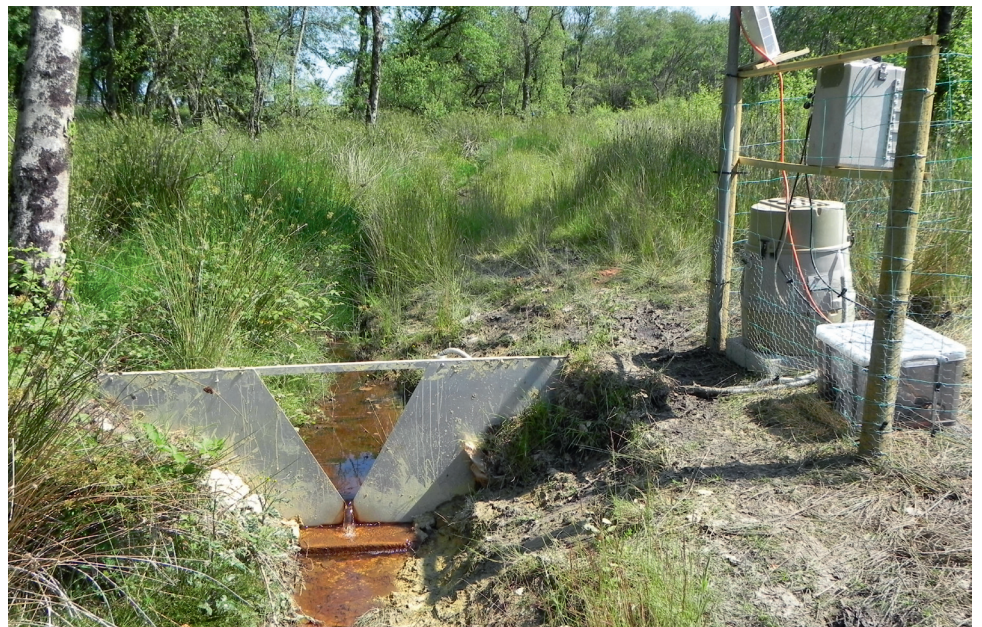
The University of Exeter is able to monitor all water entering and leaving the enclosed beaver site, showing how the new ponds that are formed by the dams the animals build store and clean the water
